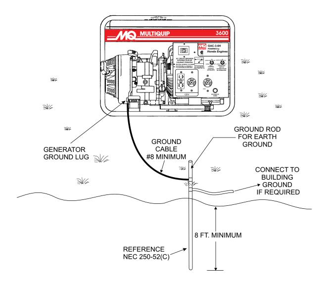
**Figure 2. Generator Grounding**
